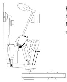
Fine adjustments to the spring roller should only be made by carefully bending the wire of the contact spring. Repeatedly bending the wire beside the screw, or at the right angle, can lead to the wire breaking.
